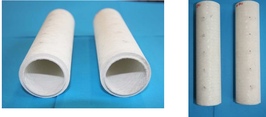
Figure 59: WHIPOX liners manufactured by DLR for transpiration cooling tests at TUM
