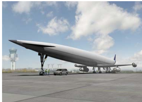
Figure 32 : LAPCAT-A2: outcome of LAPCAT I project for civil Mach 5 transport (courtesy REL)
