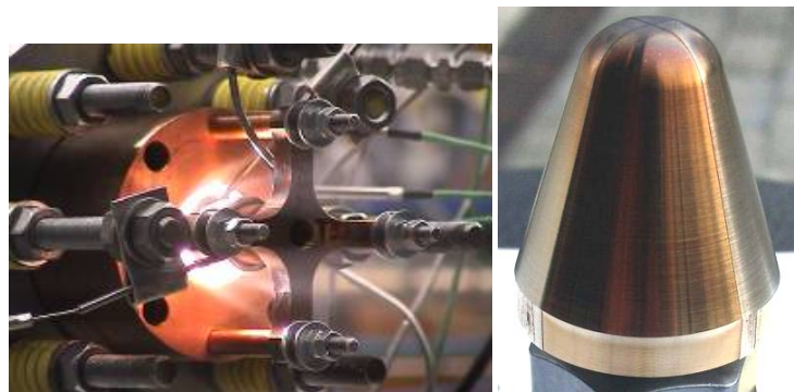
Figure 63: Inconel material samples during hot fire experiment and after test time of 300 s
