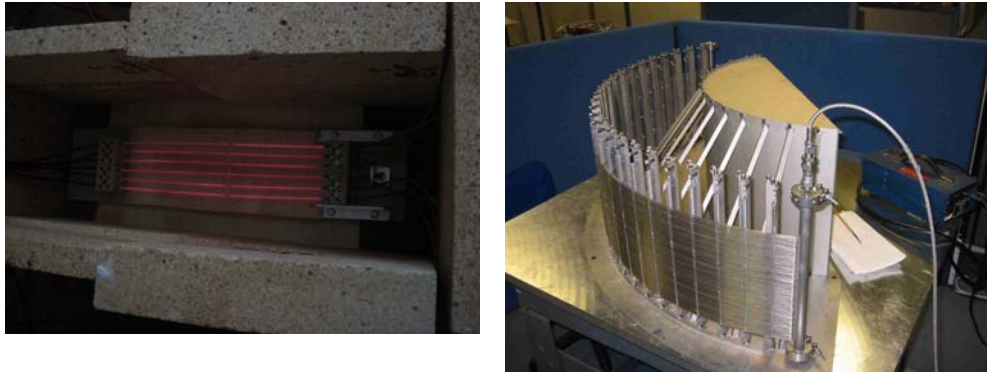
Figure 14 Left: Oxidation testing of Inconel 718 tubes, right: completed pre-cooler module in assembly fixture during pressure testing.
